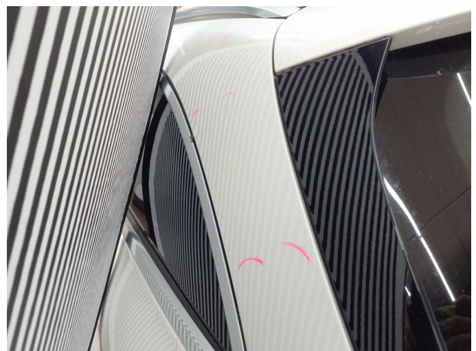
Damage 6: Body: Body - Damage by hail - Cost estimate required
