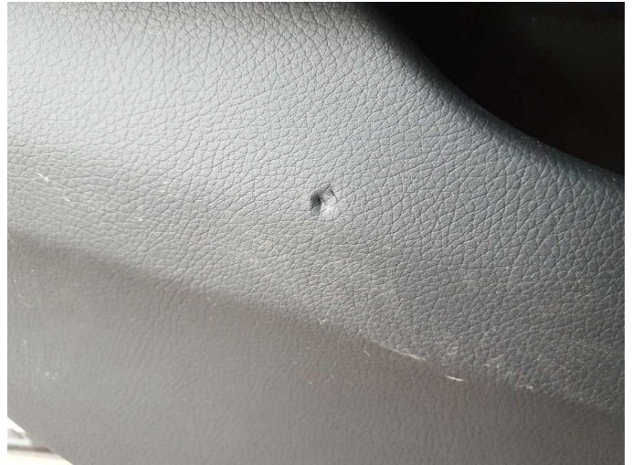
Damage 2: Trim / covers: Door trim - front left side - Damaged - Smart repair
