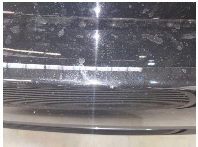
Damage 9: Rear bumper: Rear bumper - Scratch(es) - Paint
