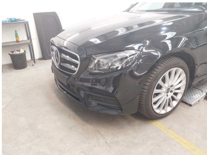
Damage 10: Front bumper: Front bumper - Scratched - Paint
