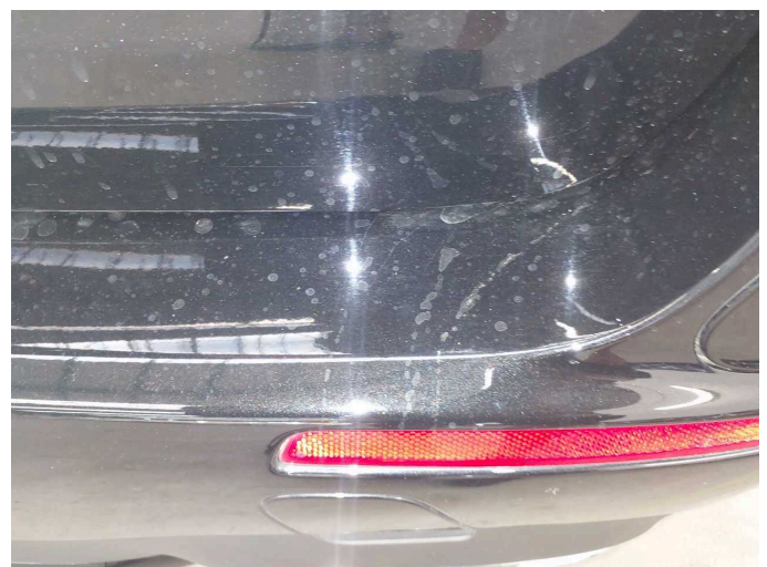
Damage 9: Rear bumper: Rear bumper - Scratch(es) - Paint
