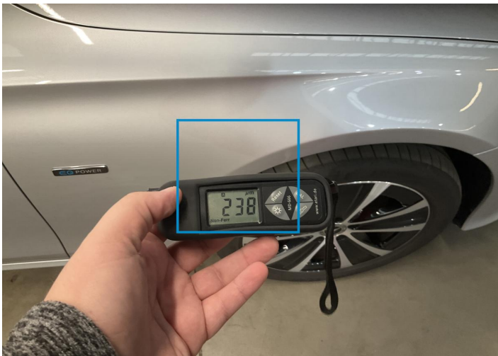
1. Fender / Front Right Paint / Poor Previous Repair -
