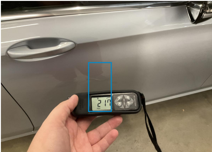
3. Door / Front Right Paint / Poor Previous Repair -
