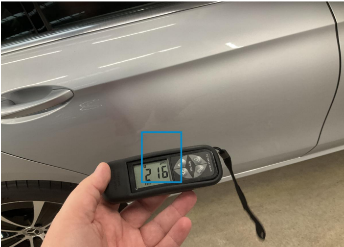
4. Door / Back Right Paint / Poor Previous Repair -
