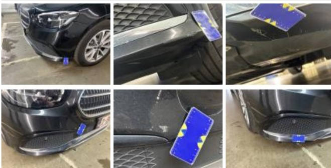
Bumper F, Scratch(es), Repair and paint (complete)
