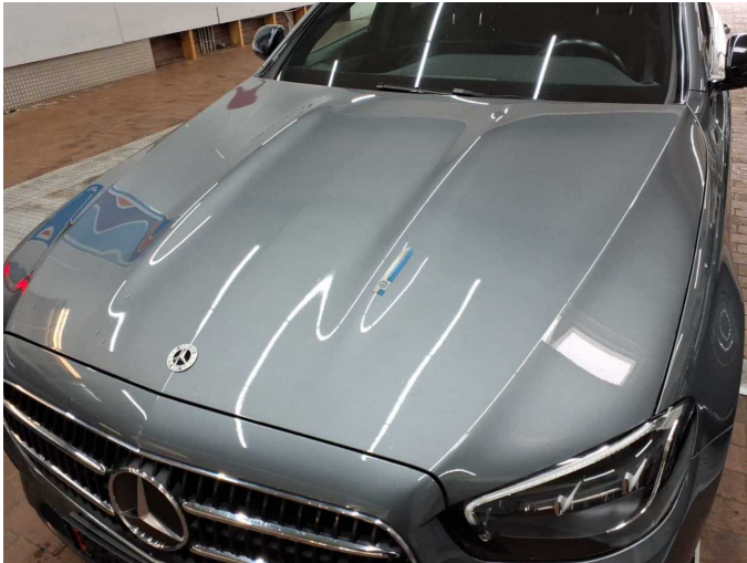
Damage 1: Bonnet: Bonnet - dent(s) - Smart repair
