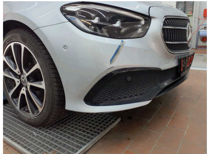
Damage 8: Front bumper: Front bumper - Scratch(es) - Paint
