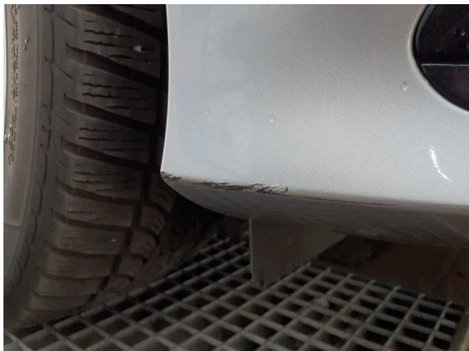
Damage 8: Front bumper: Front bumper - Scratch(es) - Paint
