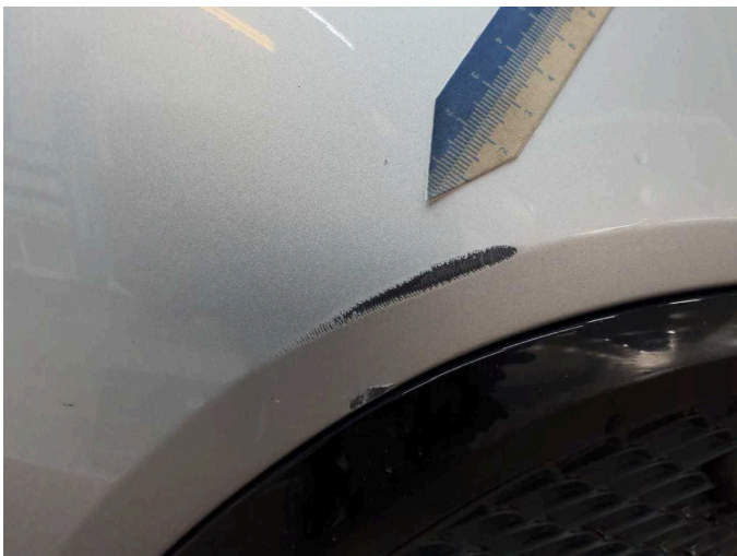
Damage 8: Front bumper: Front bumper - Scratch(es) - Paint
