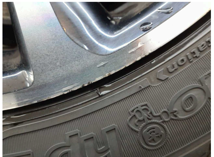
Damage 6: Wheel / tyres: Alloy rim - front right side - Scratch(es) - Loss in value
