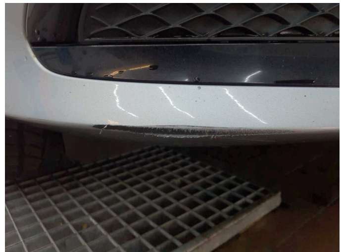
Damage 8: Front bumper: Front bumper - Scratch(es) - Paint
