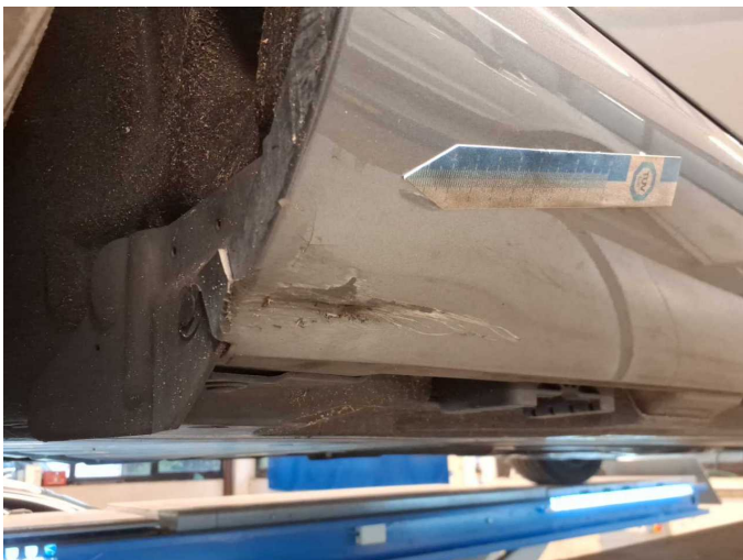
Damage 4: Sill - right side: Trim - Deformed - Replace
