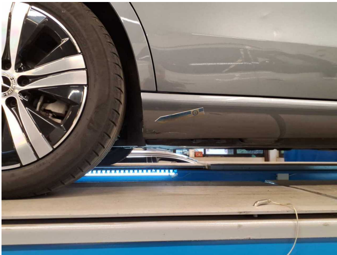
Damage 4: Sill - right side: Trim - Deformed - Replace
