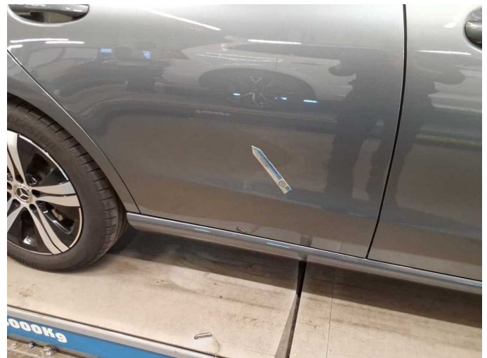
Damage 3: Door - rear right side: Door - Dent / paintcoat damage - Repair and paint
