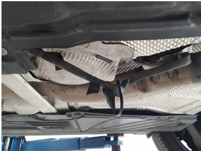
Damage 1: Exhaust system: Exhaust system (Kabel lose) - Differs from the original configuration - Un- / install
