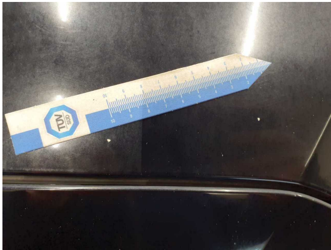
Damage 11: Bonnet: Bonnet - Stone chips - Paint
