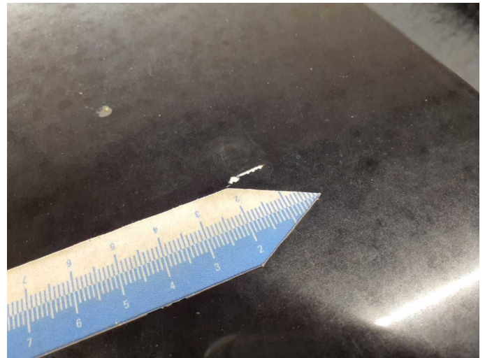
Damage 11: Bonnet: Bonnet - Stone chips - Paint
