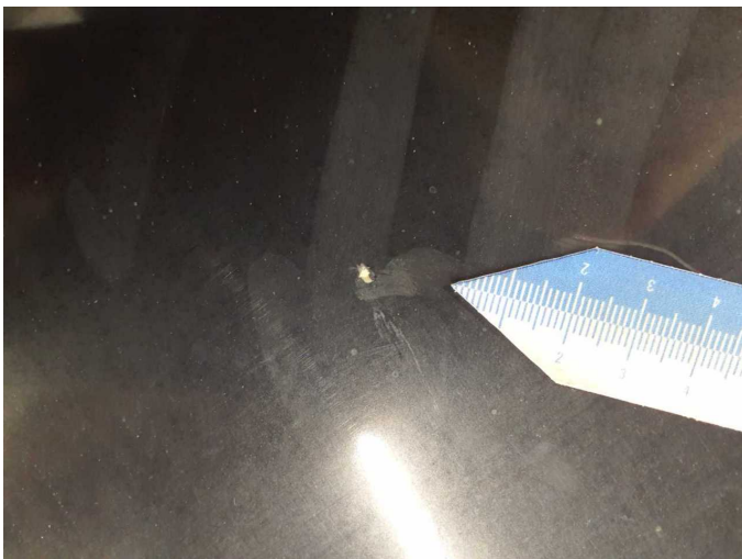
Damage 11: Bonnet: Bonnet - Stone chips - Paint
