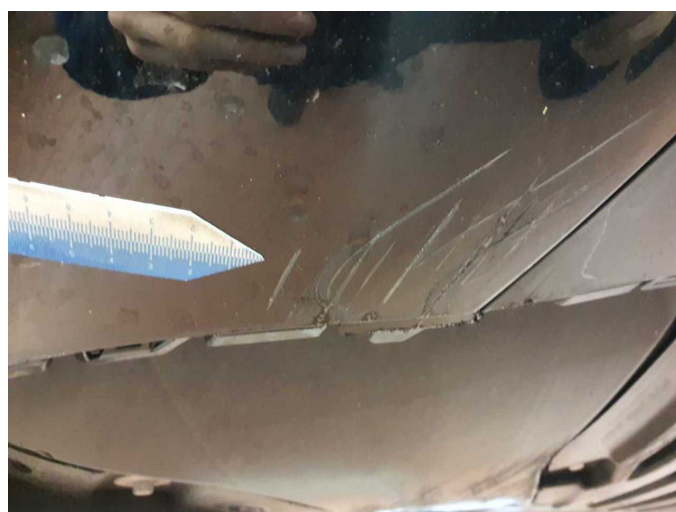
Damage 10: Front bumper: Front bumper - Scratched - Paint
