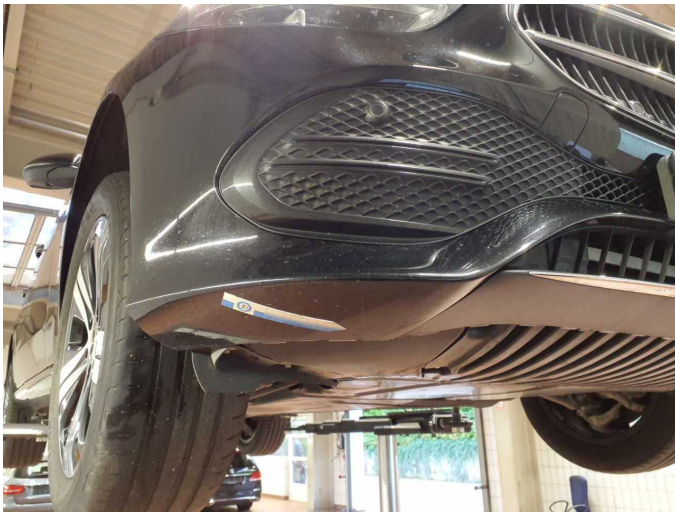
Damage 10: Front bumper: Front bumper - Scratched - Paint
