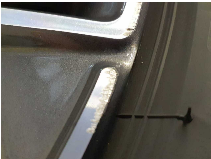
Damage 7: Wheel / tyres: Alloy rim - rear right side (Materialabtrag) - Damaged - Loss in value
