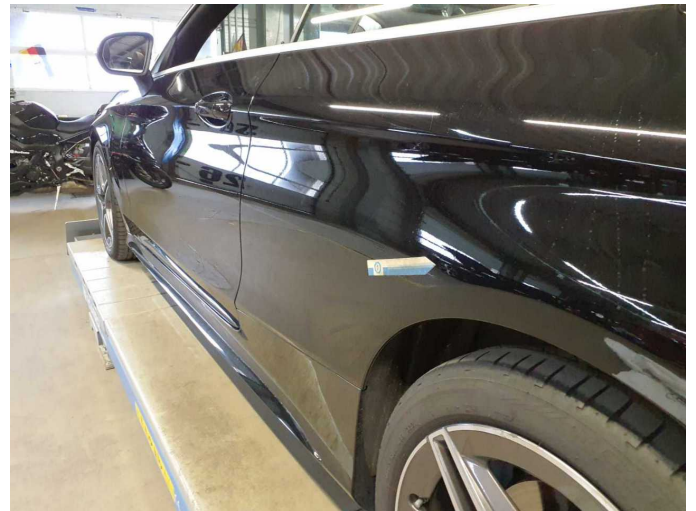
Damage 4: Side panel - rear left side: Side panel (Kratzer) - Stone chips - Smart repair
