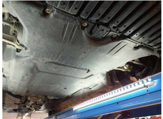
Damage 2: Body: Underbody panelling - Scratched - Replace
