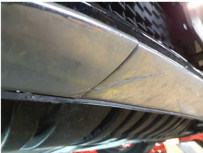
Damage 6: Front bumper: Spoiler (ZIERL M STOSSF V) - Scratched - Replace
