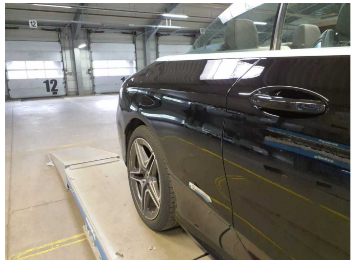
Damage 12: Side panel - rear right side: Side panel (verformt, wellig, Orangenhaut) - Unprofessionally repaired - Repair and paint
