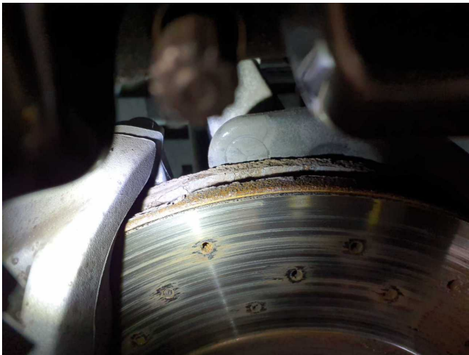
Damage 9: Braking system: Brake discs - front (Tragbild mangelhaft, Rostrand) - Corrosion - Replace
