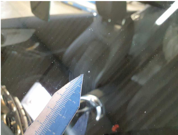
Damage 14: Vehicle glazing: Windscreen (Sandstrahleffekt) - Stone chips - Replace
