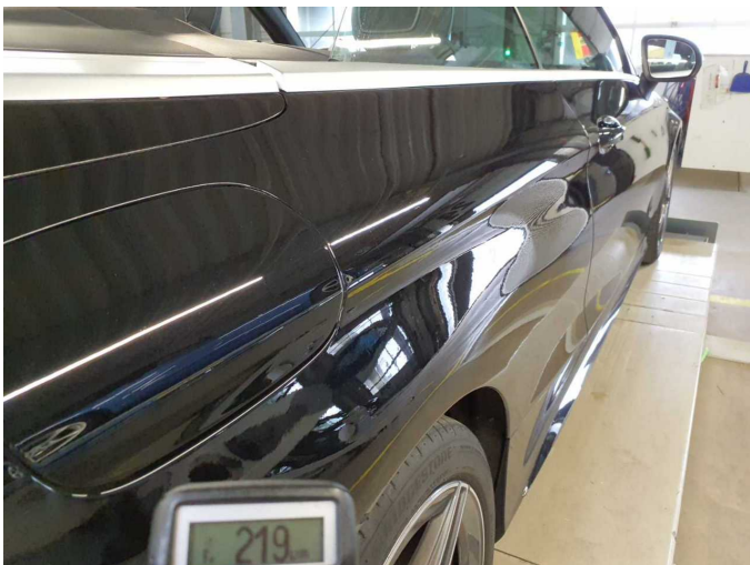
Repainting 1: Side panel - rear right side
