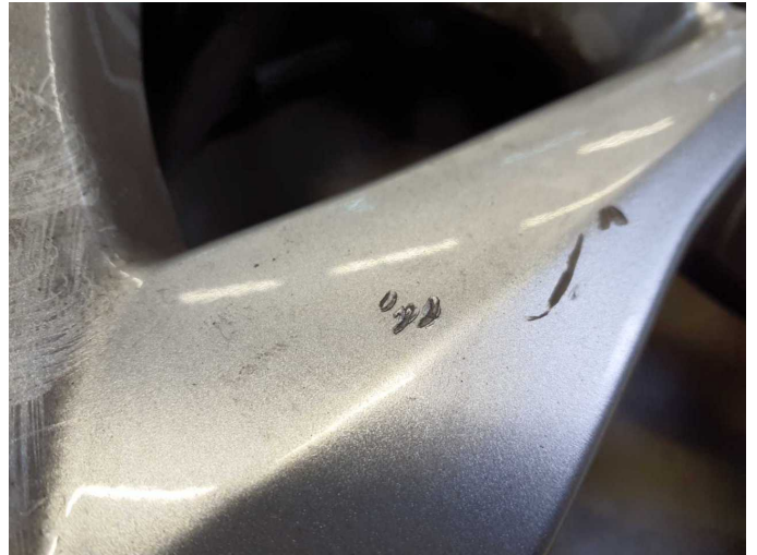
Damage 5: 2nd wheel set: 1 alloy rim (Materialabtrag) - Damaged - Loss in value
