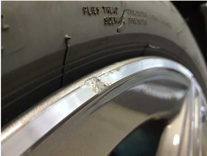
Damage 13: Wheel / tyres: Alloy rim - rear left side (Materialabtrag) - Damaged - Replace
