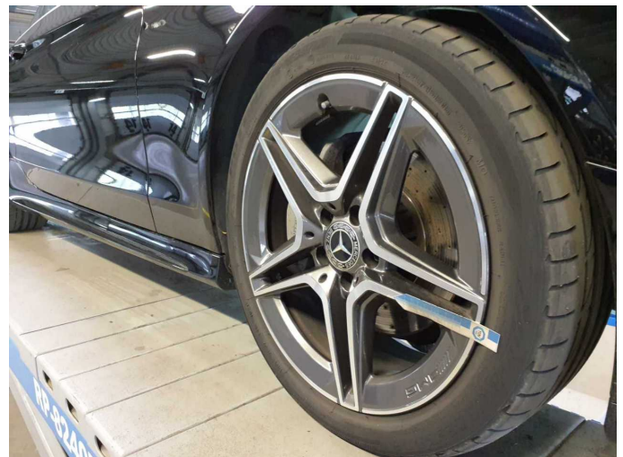
Damage 8: Wheel / tyres: Alloy rim - front right side (Materialabtrag) - Damaged - Loss in value
