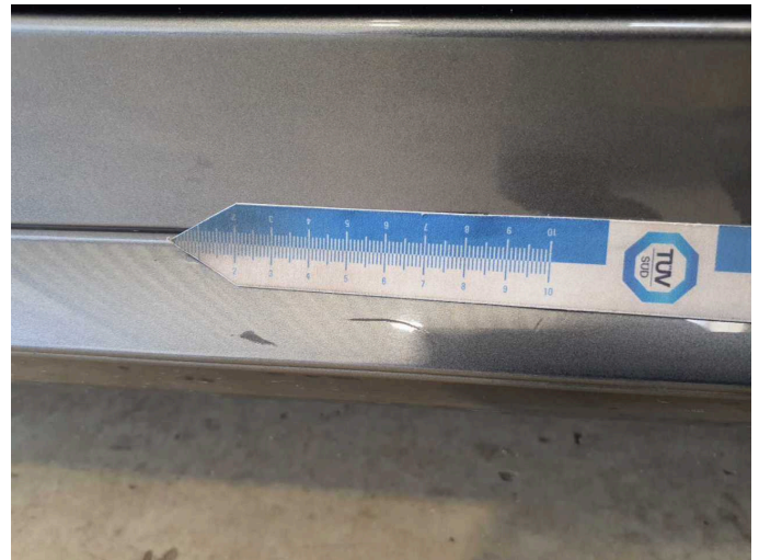
Damage 6: Sill - right side: Trim - Scratched - Smart repair
