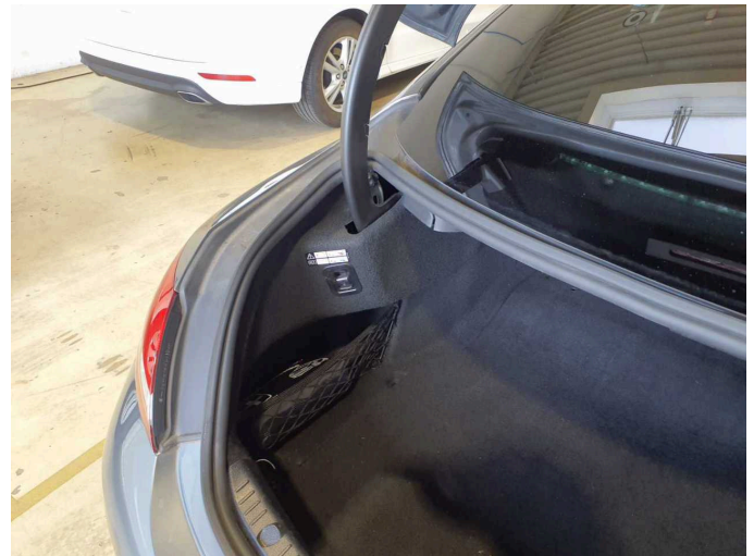
Damage 2: Trim / covers: Cargo area - lining -left side - Loose - Un- / install
