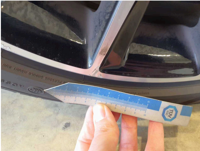
Damage 9: Wheel / tyres: Alloy rim - rear right side - Scratch(es) - Loss in value
