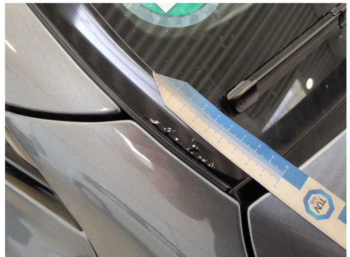
Damage 7: Roof: Cowl - right side - Corrosion - Replace
