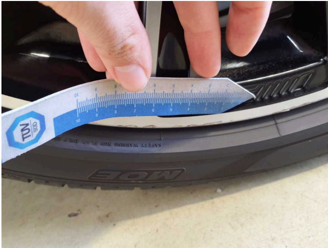
Damage 10: Wheel / tyres: Alloy rim - front left side - Scratch(es) - Measure
