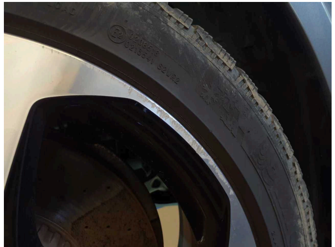
Wear and tear 2: Wheel / tyres: Alloy rim - front right side - Scratched - No deduction
