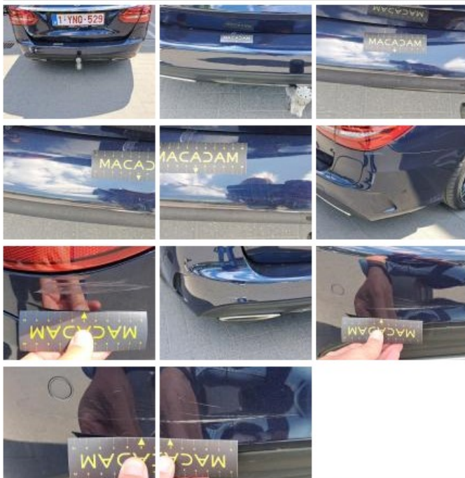
Wing RR, Dent(s) and scratch(es), Repair and paint (complete)
