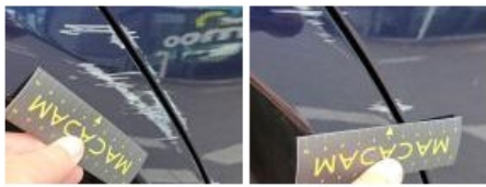
Door RR, Scratch(es), Repair and paint (complete)
