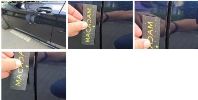
Wing RL, Dent(s) and scratch(es), Acceptable
