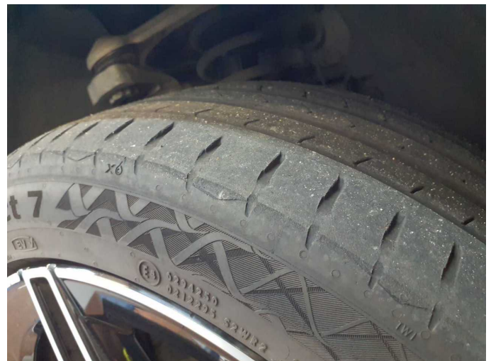
Damage 5: Wheel / tyres: Tyre - front - Worn - Replace
