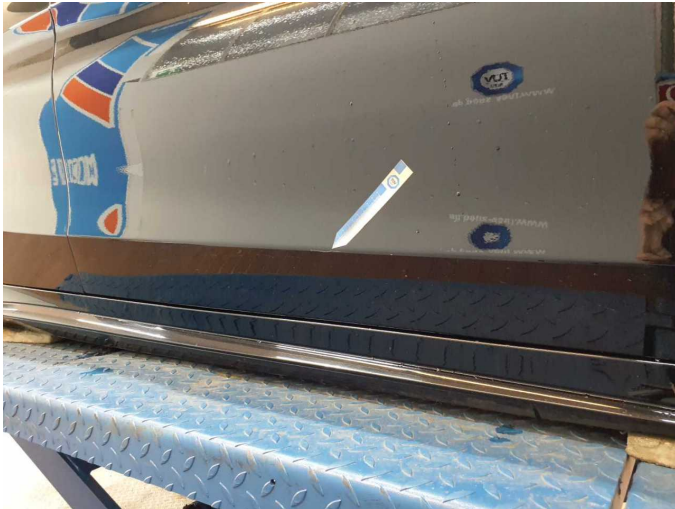
Damage 3: Door - front right side: Door - Scratched - Loss in value
