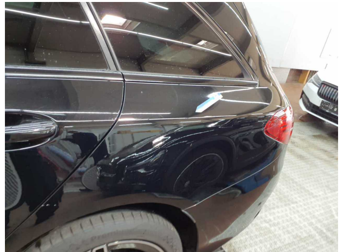
Damage 8: Side panel - rear left side: Side panel (+ Krater) - dent(s) - Paint
