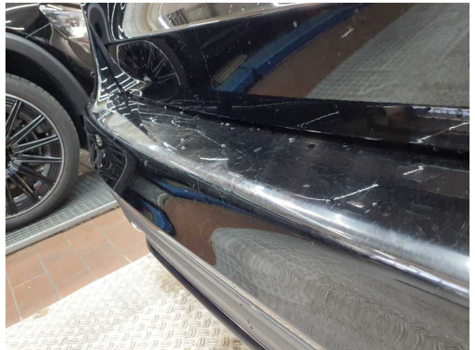
Damage 11: Rear bumper: Rear bumper (+ Leicht Delle) - Scratched - Repair and paint
