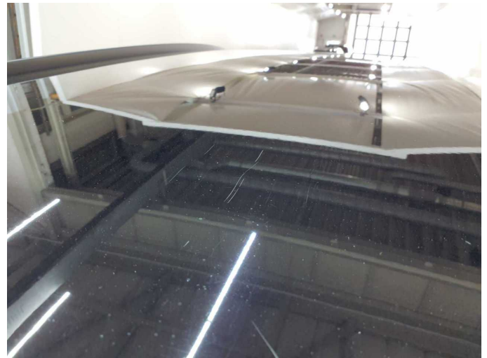
Damage 13: Roof: Roof - Scratched - Lacquer
