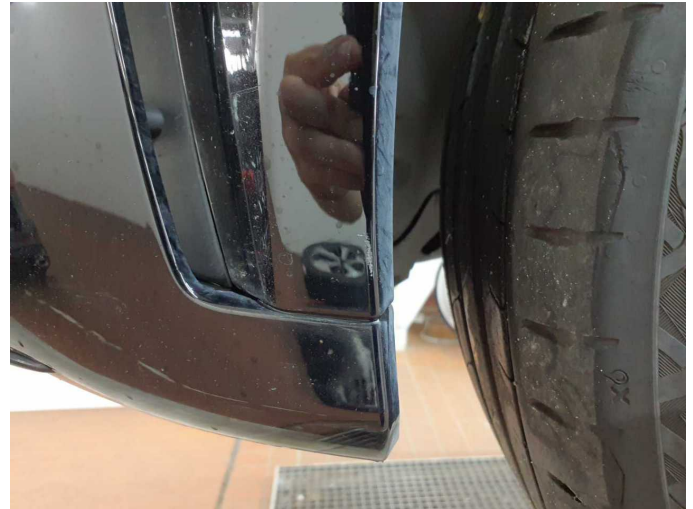
Damage 14: Front bumper: Front bumper (Inklusive Blenden erneuern) - Scratched - Repair and paint
