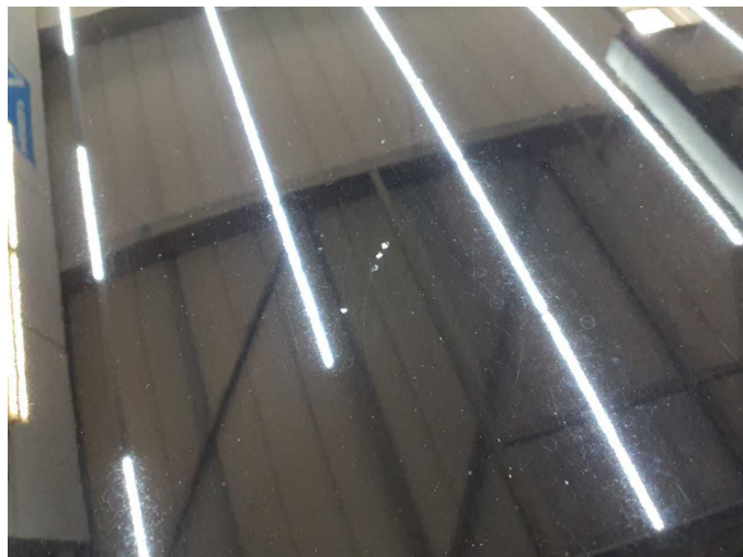
Damage 10: Bonnet: Bonnet (+ Krater) - Stone chips - Paint
