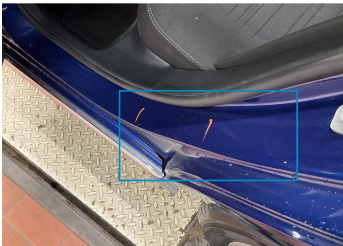
3. Pillar / Back Left Bodywork / Dent / Dent -
