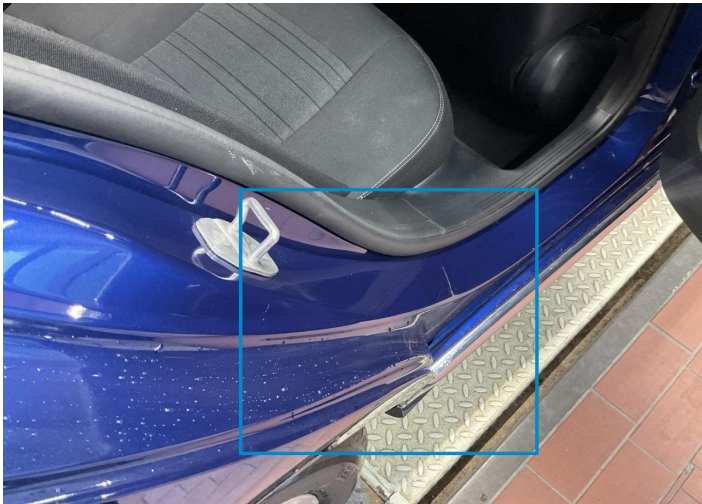
10. Pillar / Back Right Paint / Scratch / Scuff -
