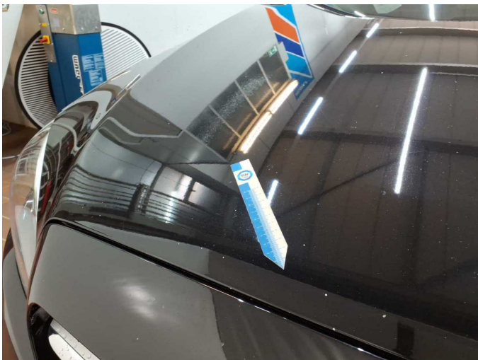
Damage 4: Bonnet: Bonnet - Stone chips - Paint
