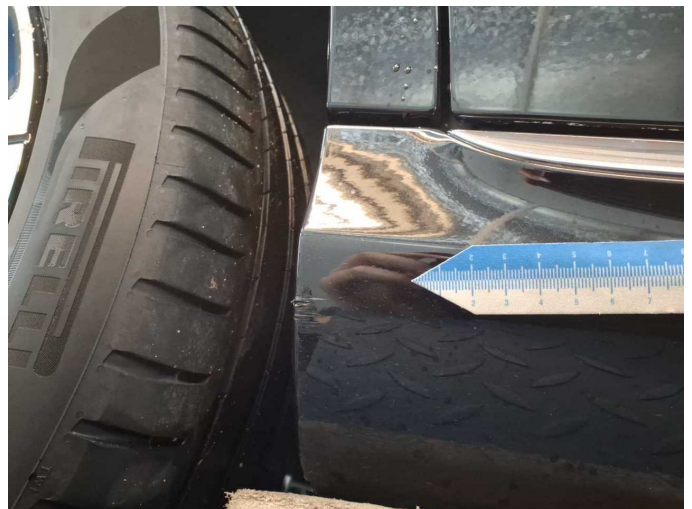
Damage 2: Sill - right side: Sill - Scratched - Smart repair
