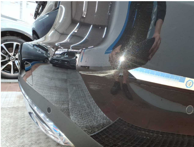
Damage 5: Rear bumper: Rear bumper - Scratch(es) - Paint
