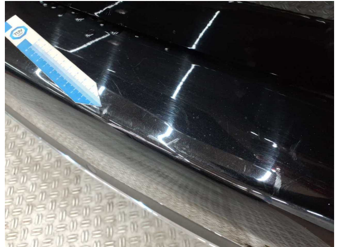
Damage 5: Rear bumper: Rear bumper - Scratch(es) - Paint
