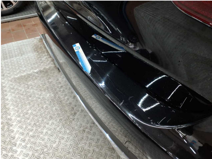
Damage 5: Rear bumper: Rear bumper - Scratch(es) - Paint
