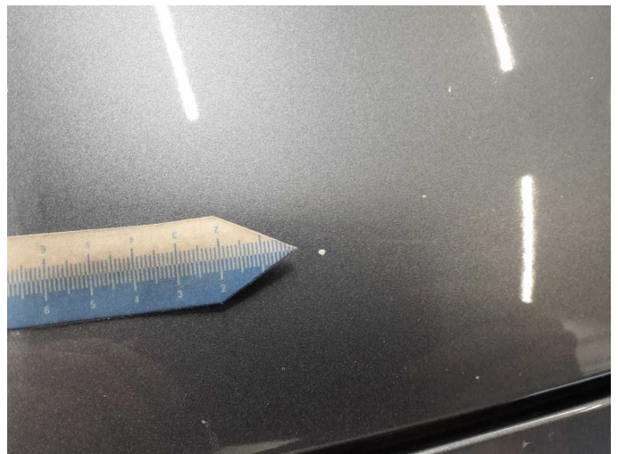
Damage 7: Bonnet: Bonnet - Stone chips - Paint
