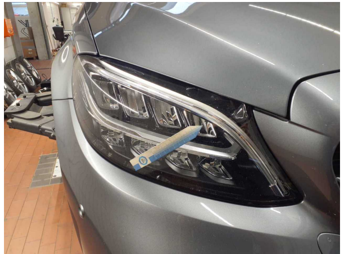
Damage 6: Headlight: Headlight - right side - Stone chips - Loss in value
