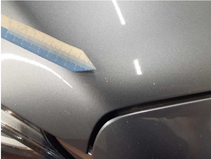
Damage 7: Bonnet: Bonnet - Stone chips - Paint
