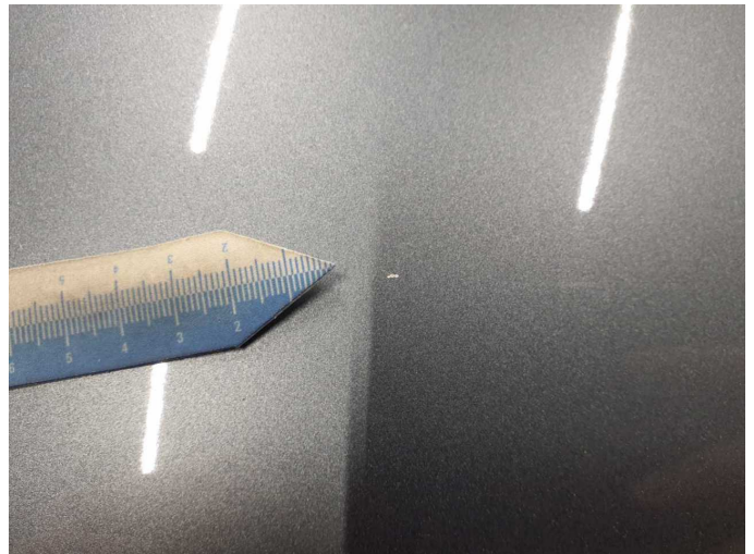
Damage 7: Bonnet: Bonnet - Stone chips - Paint
