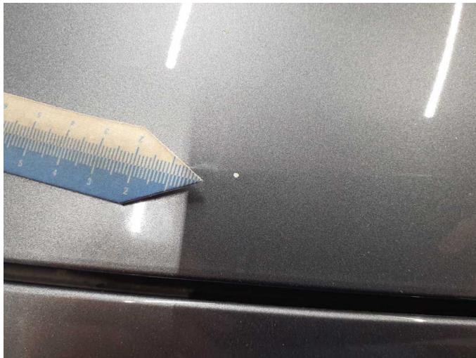
Damage 7: Bonnet: Bonnet - Stone chips - Paint
