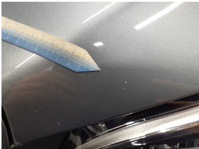
Damage 7: Bonnet: Bonnet - Stone chips - Paint
