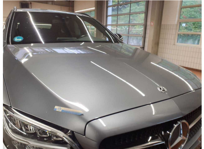
Damage 7: Bonnet: Bonnet - Stone chips - Paint
