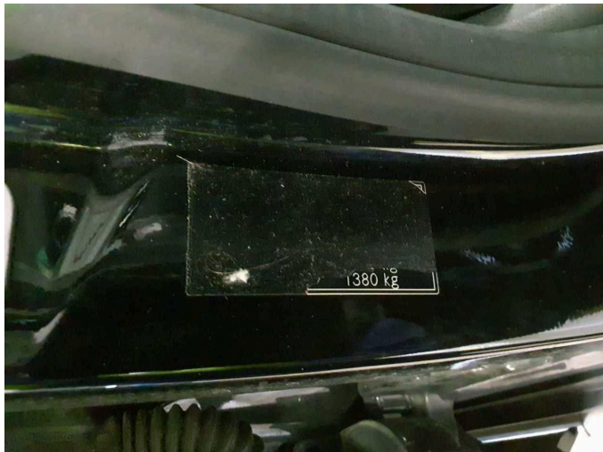
Damage 3: Body: Identification plate - Missing - Replace
