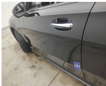
Door Front Left // Repair & Painting-scratch + dent
