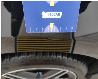
Wing Rear Right // Repair & Painting-scratch + dent
