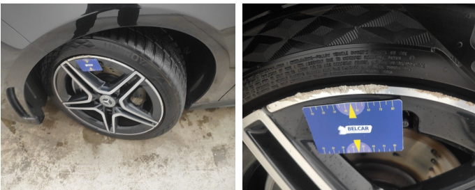
Wheel Two Tone Front Left // Repair-scratch
