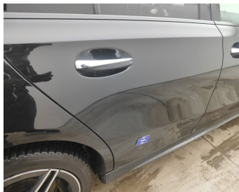
Door Rear Right // Repair & Painting-scratch + dent
