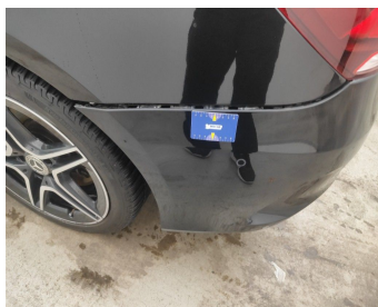
Bumper Rear // Replace & Painting-cracked
