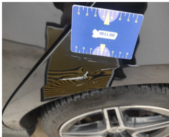
Wing Rear Left // Repair & Painting-scratch + dent
