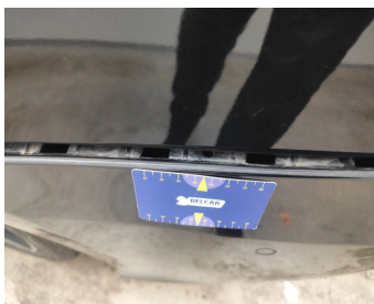
Bumper Rear // Replace & Painting-cracked
