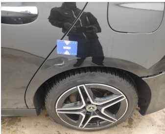
Wing Rear Left // Repair & Painting-scratch + dent
