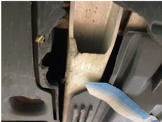
Damage 2: Front axle: Axles / undercarriage (Rahmen) - Damaged - Replace
