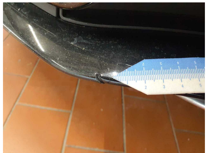
Damage 11: Front bumper: Front bumper - Broken / torn - Replace
