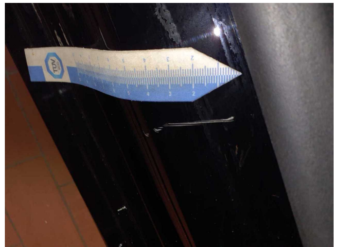
Damage 4: Side panel - rear right side: Sill - Scratched - Smart repair
