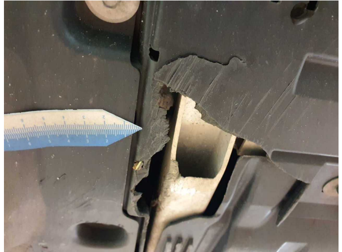
Damage 8: Body: Underbody panelling - Broken / torn - Replace
