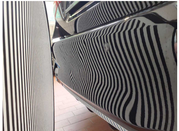
Damage 10: Rear bumper: Rear bumper - Deformed - Replace
