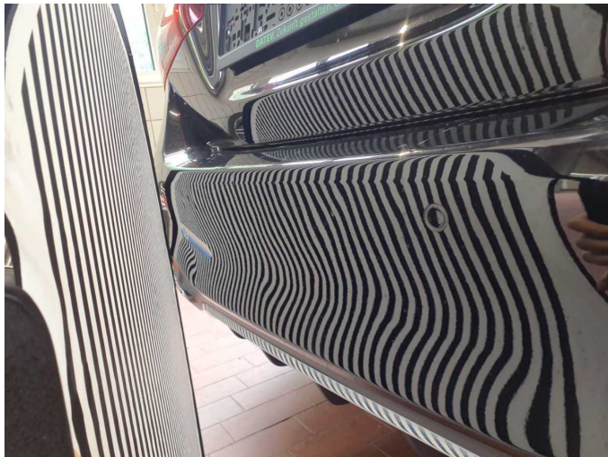
Damage 10: Rear bumper: Rear bumper - Deformed - Replace
