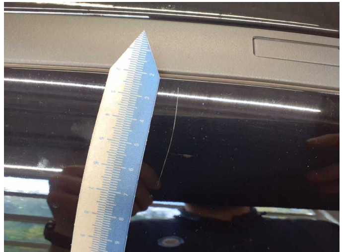
Damage 9: Roof: Roof rail - left side - Scratch(es) - Paint
