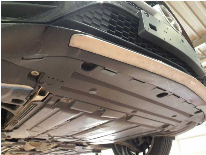
Damage 8: Body: Underbody panelling - Broken / torn - Replace
