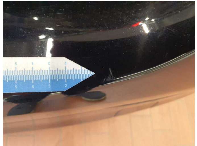
Damage 10: Rear bumper: Rear bumper - Deformed - Replace
