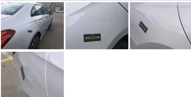
Wing RR, Dent(s), Repair and paint (complete)
