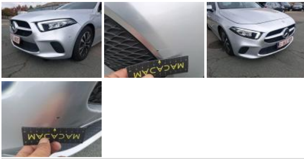
Sill trim L, Dent(s) and scratch(es), Repair and paint (complete)
