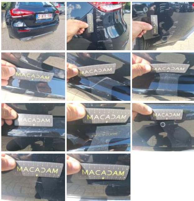
Rear light L, Scratch(es), Replace
