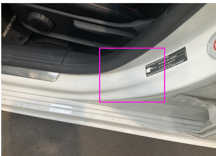
3. B Pillar / Center Left Bodywork / Dent / Dent -
