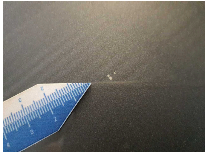
Damage 3: Bonnet: Bonnet - Stone chips - Paint
