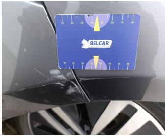
Wing Front Left // Smart Repair Medium-scratch
