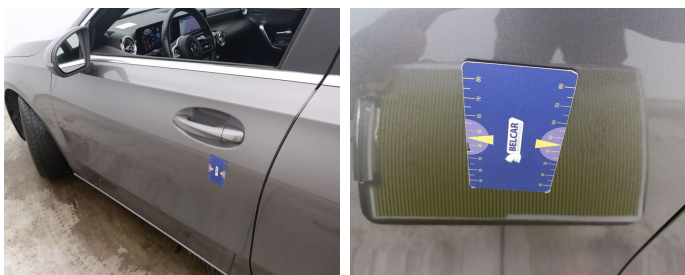
Door Front Left // Repair & Painting-scratch + dent
