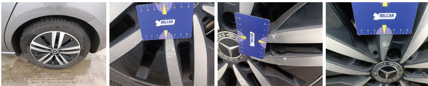
Wheel Two Tone Rear Left // Repair-Chemical reaction
