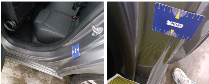
Rocker Panel Left // Smart Repair Medium-scratch + dent
