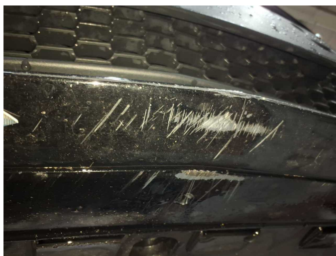
Damage 4: Front bumper: Front bumper - Scratched - Repair and paint
