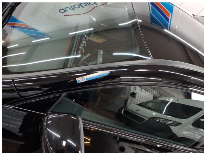
Damage 2: Roof: Roof rail - left side - Stone chips - Smart repair
