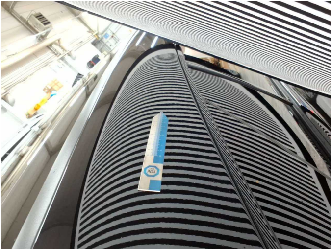
Wear and tear 6: Roof: Roof rail - right side - dent(s) - No deduction
