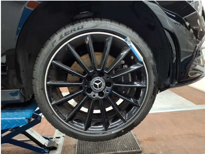
Damage 5: Wheel / tyres: Alloy rim - front right side (Materialabtrag) - Scratched - Replace
