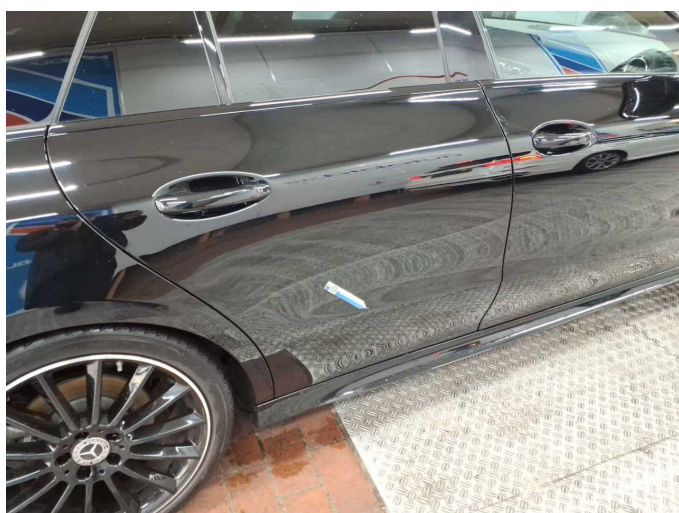
Damage 3: Door - rear right side: Door - Scratched - Paint
