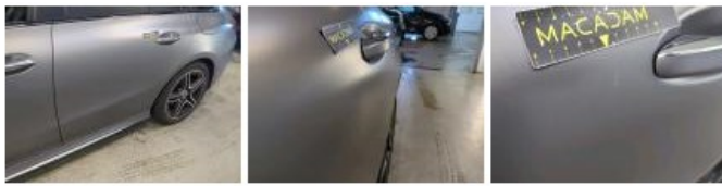
Door FL, Dent(s), Repair and paint (complete)
