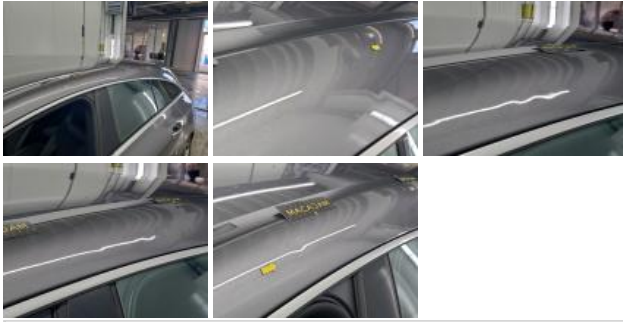
Door FL, Scratch(es), Repair and paint (partial)
