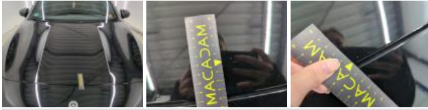
Bumper F, Scratch(es), Repair and paint (complete)
