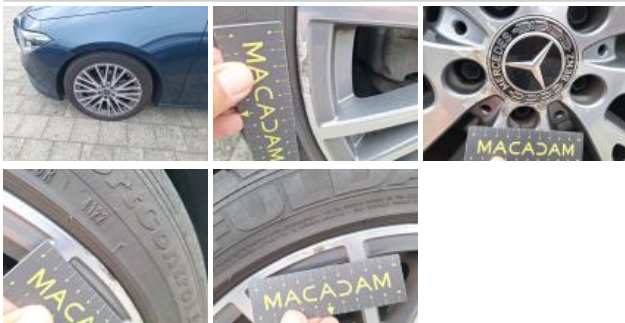
Alloy rim RL polished, Scratch(es), Repair and paint (complete)
