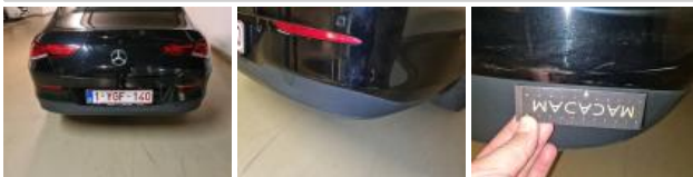
Bumper moulding R, Scratch(es), Replace
