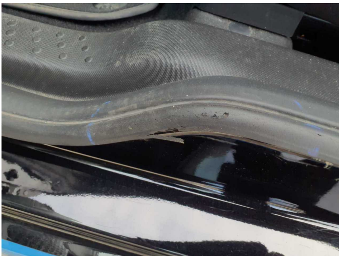
Damage 4: Body: Door seal - front left side - Broken / torn - Replace
