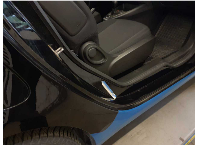
Damage 1: Side panel - rear right side: Sill (1) - dent(s) - Smart repair
