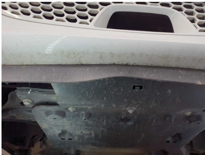
Damage 6: Front bumper: Spoiler - Deformed - Replace
