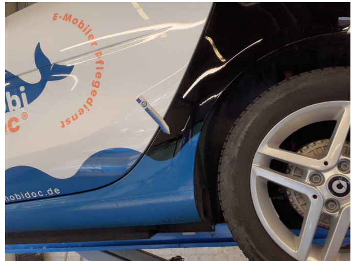
Damage 2: Side panel - rear left side: Elbow (1) - dent(s) - Smart repair
