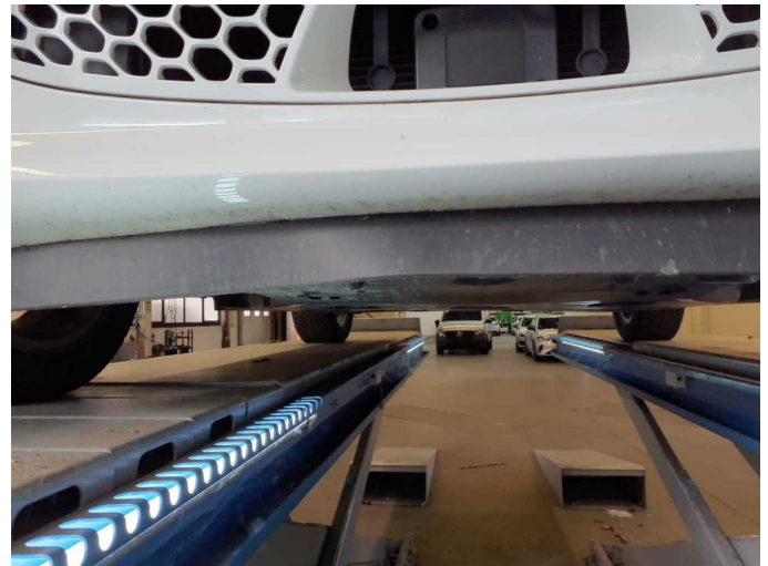
Damage 6: Front bumper: Spoiler - Deformed - Replace
