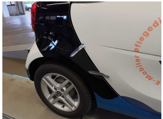
Damage 3: Side panel - rear right side: Wheel arch (+gebrauchsspuren) - dent(s) - Smart repair
