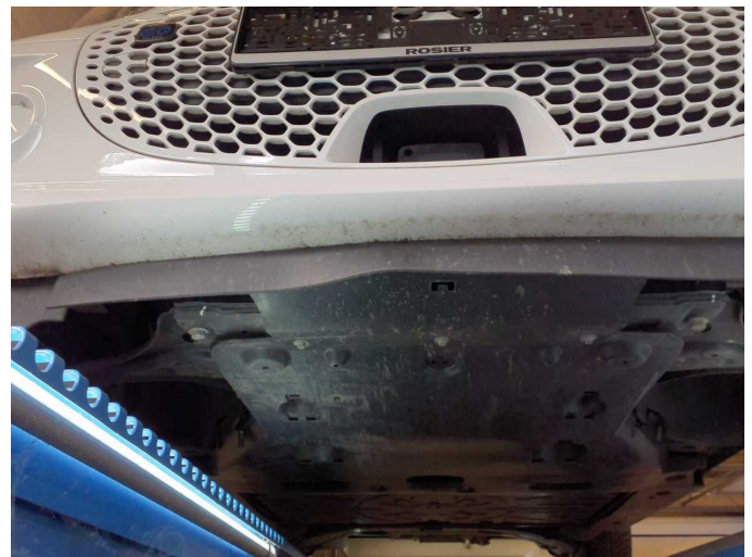
Damage 6: Front bumper: Spoiler - Deformed - Replace
