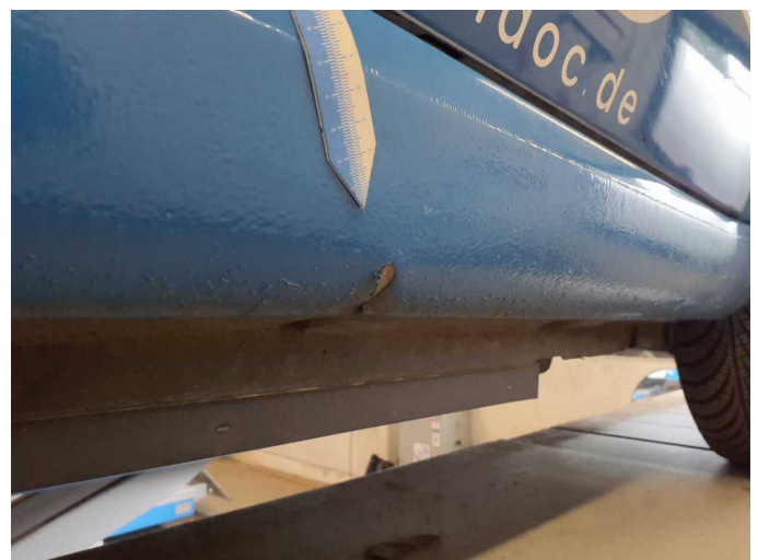
Damage 8: Sill - right side: Sill - Damaged - Repair and paint
