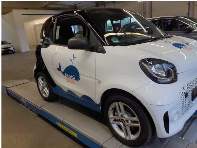
Damage 7: Body: Body - Glued / labelled - De-glue / neutralise
