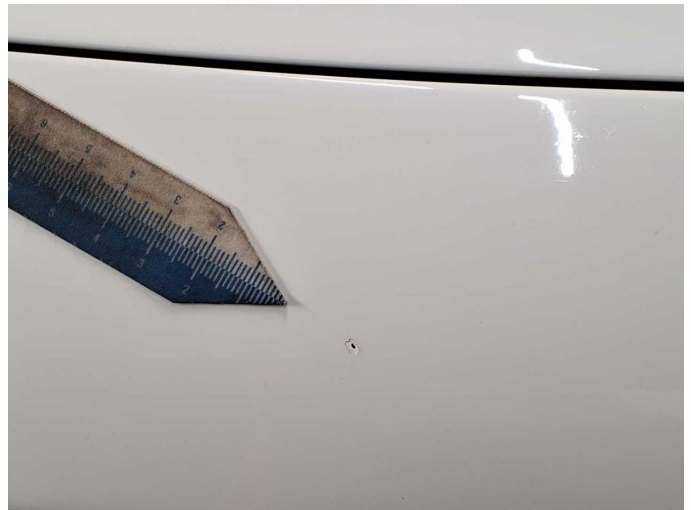
Wear and tear 5: Front bumper: Front bumper - Stone chips - Smart repair
