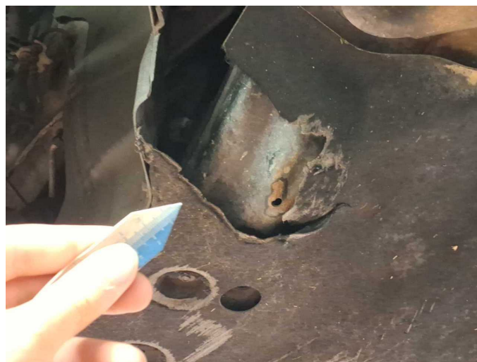
Damage 3: Body: Underbody panelling - Broken / torn - Replace
