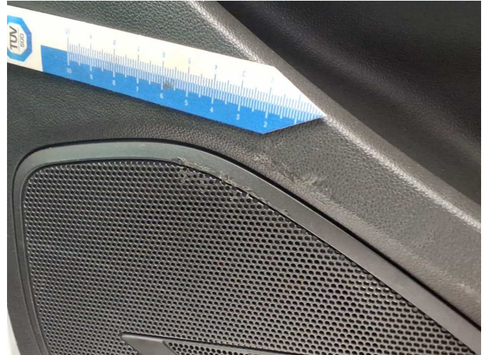
Damage 5: Trim / covers: Door trim - rear right side - Broken / torn - Replace
