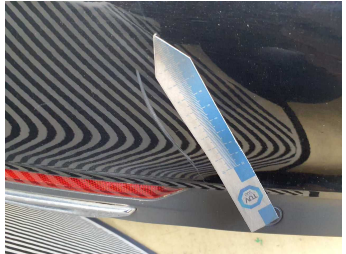
Damage 8: Rear bumper: Rear bumper - Scratch(es) - Paint
