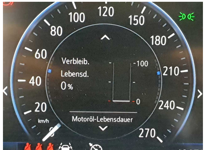
Damage 6: Misc.: Inspection / maintenance - Due - Perform
