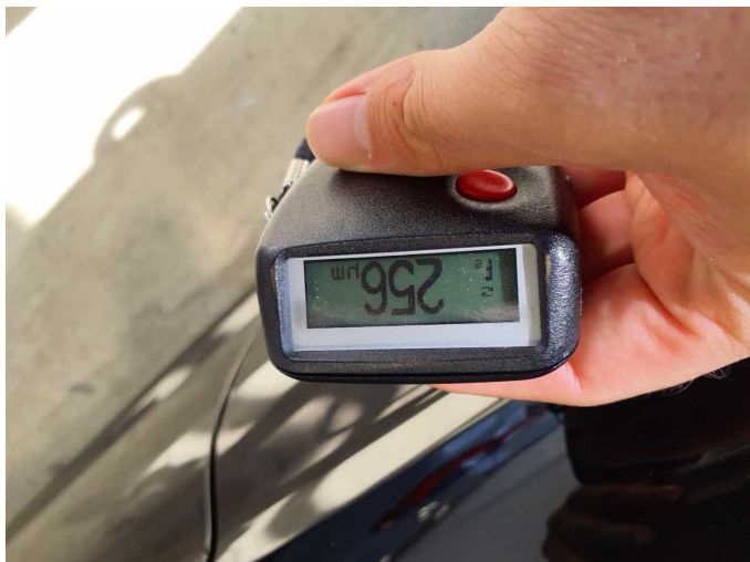
Repainting 1: Roof, Door - rear right side
