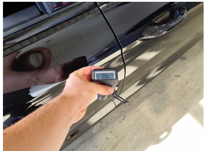
Repainting 1: Roof, Door - rear right side
