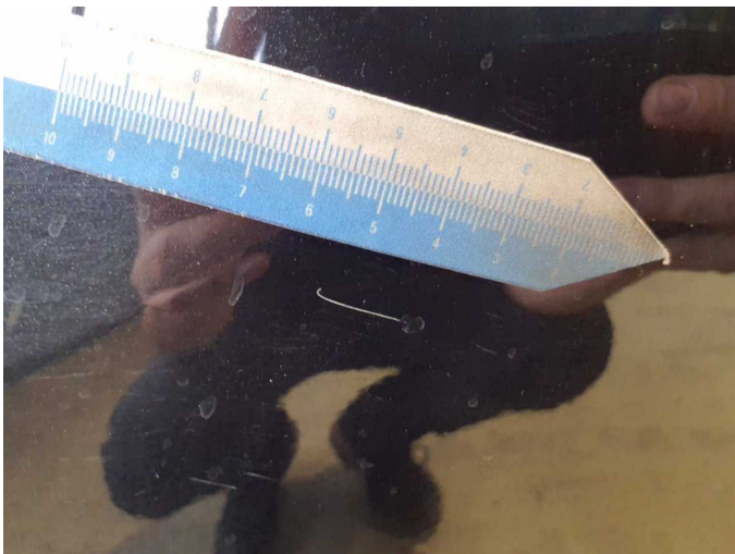
Damage 8: Rear bumper: Rear bumper - Scratch(es) - Paint
