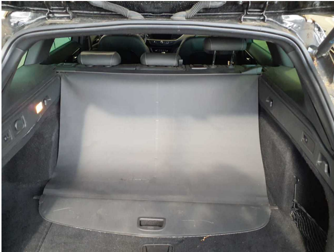
Damage 7: Interior: Boot cover / roller cover - Damaged - Replace
