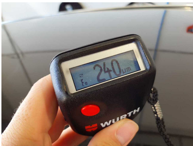
Repainting 1: Roof, Door - rear right side
