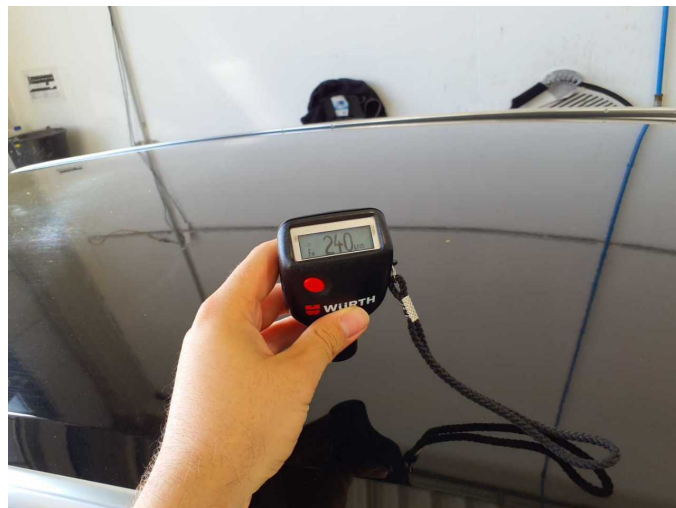
Repainting 1: Roof, Door - rear right side
