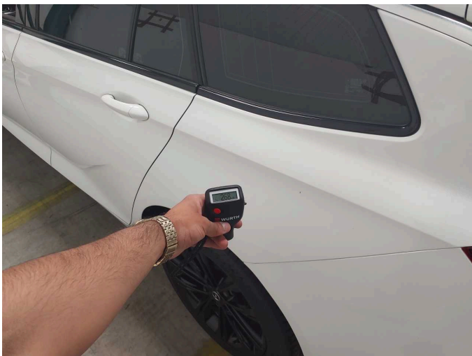
Side panel - rear left side: 268 µm
