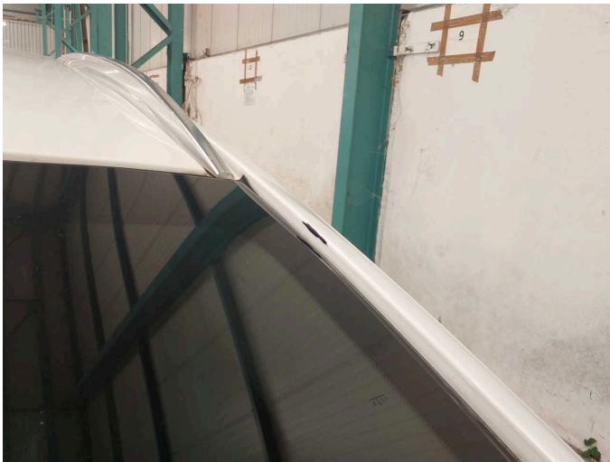
Damage 3: Roof: Roof rail - left side - Scratched - Smart repair
