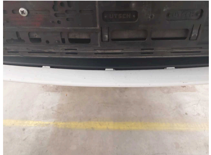
Damage 7: Front bumper: Front bumper - Dent / paintcoat damage - Repair and paint
