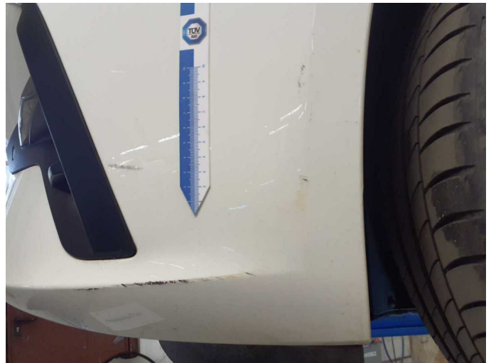
Damage 7: Front bumper: Front bumper - Scratch(es) - Paint
