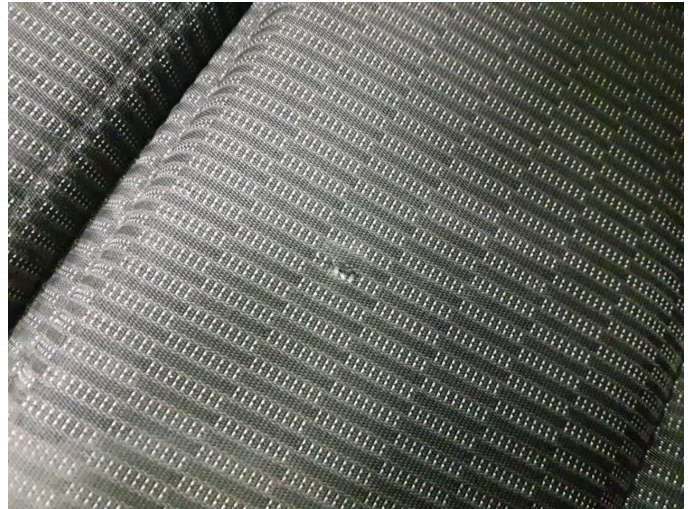
Damage 5: Seat - front: Seat cover - left side (+verschmutzt) - Holes - Smart repair
