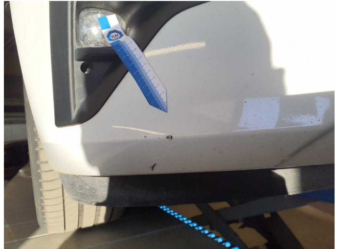
Damage 7: Front bumper: Front bumper - Scratch(es) - Paint
