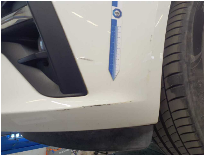
Damage 7: Front bumper: Front bumper - Scratch(es) - Paint
