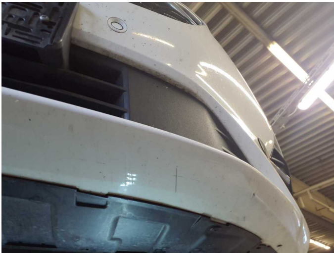
Damage 7: Front bumper: Front bumper - Scratch(es) - Paint
