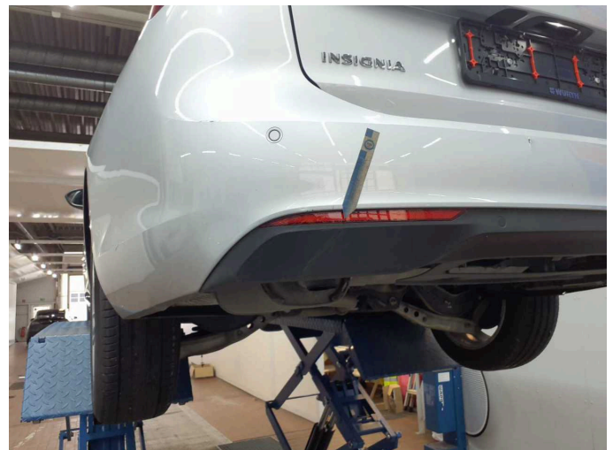
Damage 5: Rear bumper: Spoiler (+ Reflektor) - Scratched - Replace
