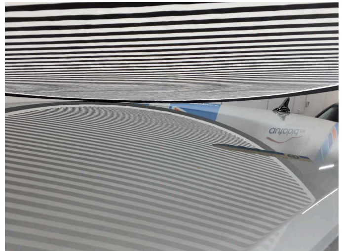
Damage 4: Roof: Roof - dent(s) - Smart repair
