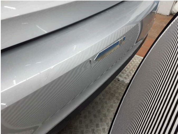
Damage 7: Rear bumper: Rear bumper - Damaged - Replace
