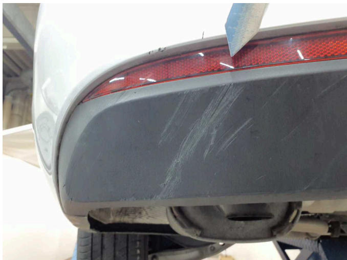
Damage 5: Rear bumper: Spoiler (+ Reflektor) - Scratched - Replace
