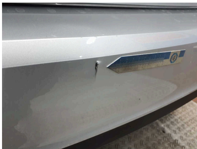
Damage 7: Rear bumper: Rear bumper - Damaged - Replace
