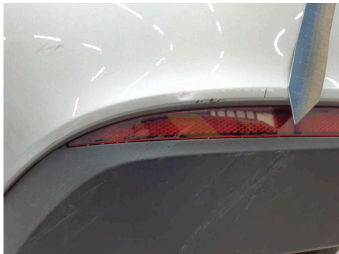
Damage 5: Rear bumper: Spoiler (+ Reflektor) - Scratched - Replace
