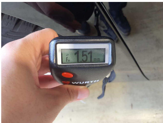
Repainting 2: Side panel - rear right side
