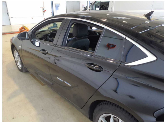
Damage 8: Door - rear left side: Door - Deformed - Repair and paint
