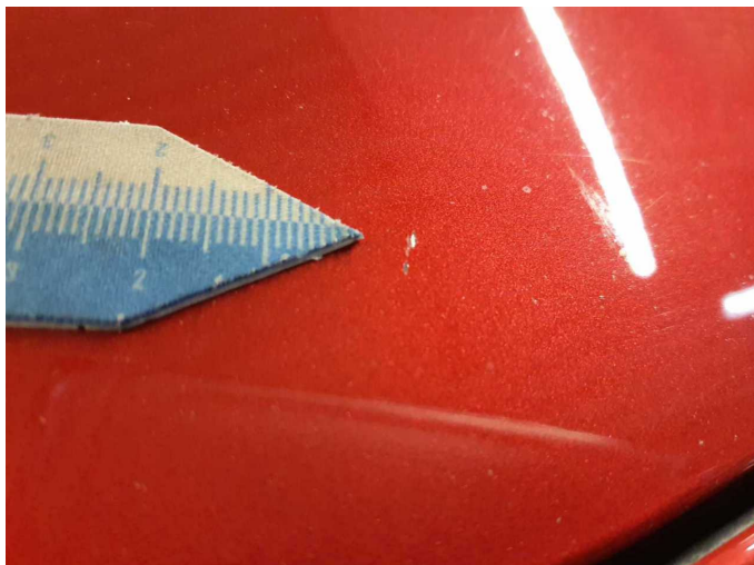
Damage 11: Bonnet: Bonnet (Kratzer/Steinschlag) - dent(s) - Repair and paint
