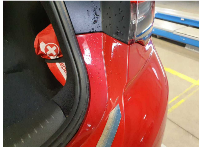
Damage 10: Rear bumper: Rear bumper - Scratched - Paint
