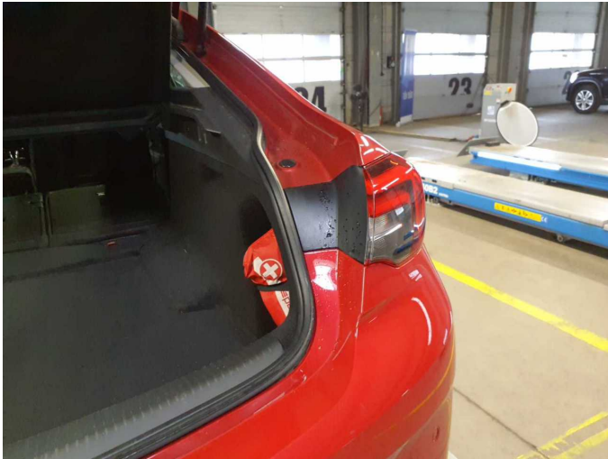
Damage 10: Rear bumper: Rear bumper - Scratched - Paint
