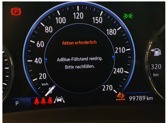
Damage 1: Instrument panel: Indicator light (AdBlue) - on - Replace
