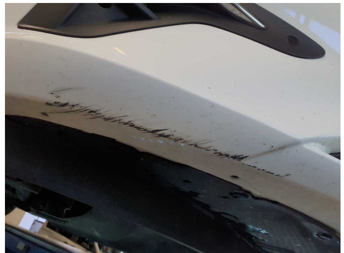
Damage 6: Front bumper: Front bumper - Scratch(es) - Paint
