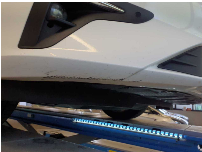
Damage 6: Front bumper: Front bumper - Scratch(es) - Paint
