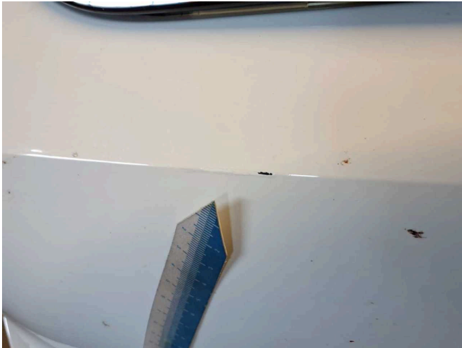
Damage 4: Front bumper: Front bumper - Scratch(es) - Paint
