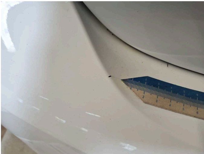
Damage 3: Rear bumper: Rear bumper - Scratch(es) - Paint
