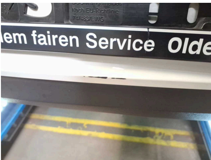
Damage 3: Rear bumper: Rear bumper - Scratch(es) - Paint
