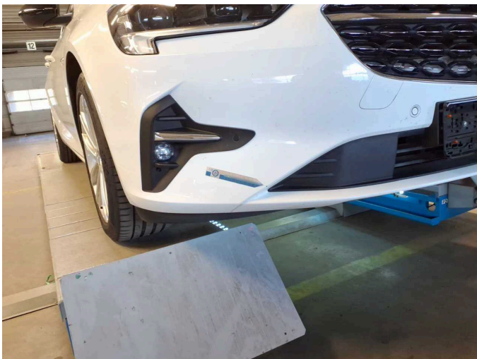
Damage 4: Front bumper: Front bumper - Scratch(es) - Paint
