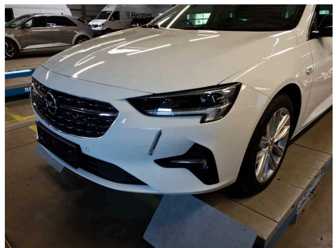
Damage 4: Front bumper: Front bumper - Scratch(es) - Paint
