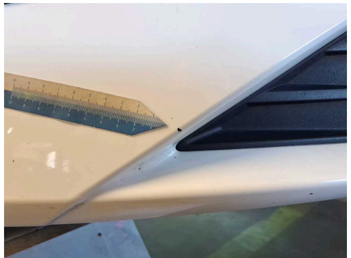
Damage 4: Front bumper: Front bumper - Scratch(es) - Paint
