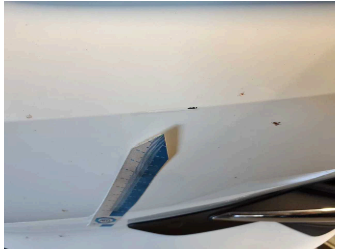
Damage 4: Front bumper: Front bumper - Scratch(es) - Paint
