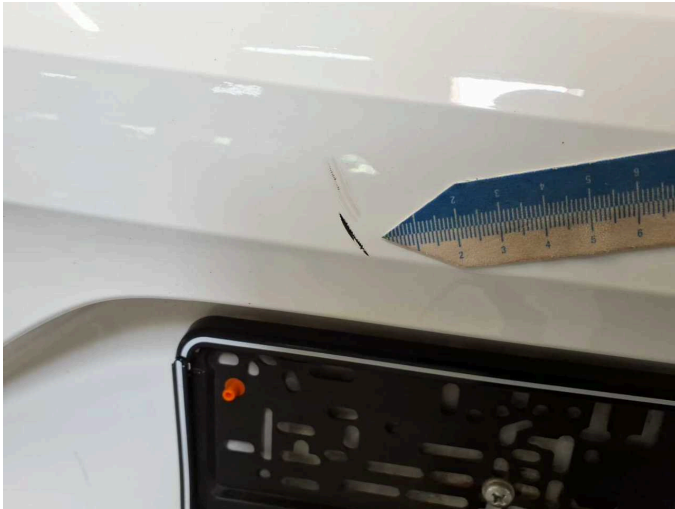
Damage 3: Rear bumper: Rear bumper - Scratch(es) - Paint
