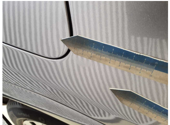
Damage 2: Side panel - rear right side: Side panel (Wellig, stellenweise matt, Spachtel eingefallen) - Unprofessionally repaired - Repair and paint
