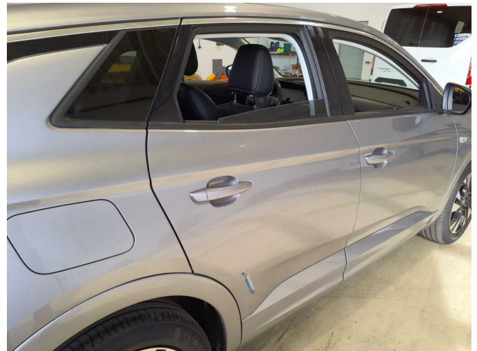
Damage 3: Door - rear right side: Door (Wellig, Spachtel eingefallen) - Unprofessionally repaired - Repair and paint
