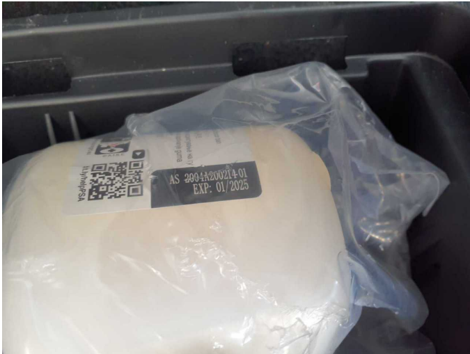
Damage 1: Equipment: Tirefit filler - Expired - Replace
