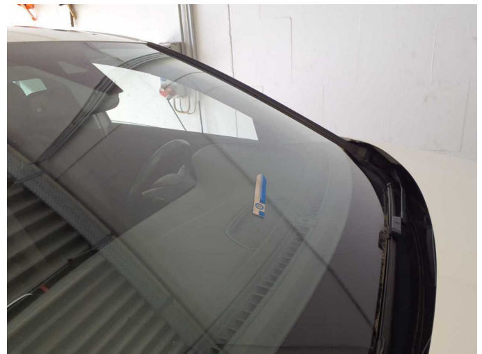
Wear and tear 1: Vehicle glazing: Windscreen with lane departure assistant - Stone chips - No deduction
