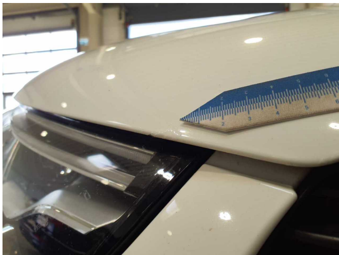
Damage 8: Bonnet: Bonnet - Corrosion - Repair and paint
