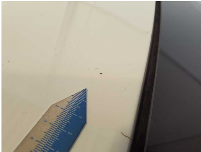
Damage 4: Roof: Roof - Stone chips - Smart repair
