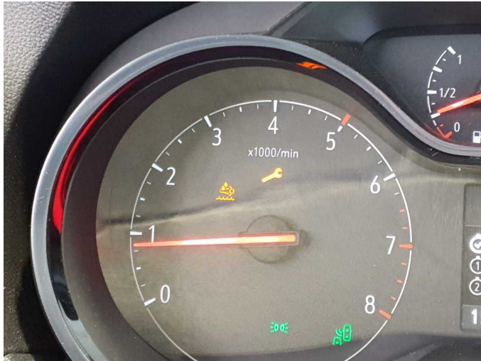
Damage 7: Instrument panel: Indicator light (Abgasnachbehandlung) - on - Perform diagnosis
