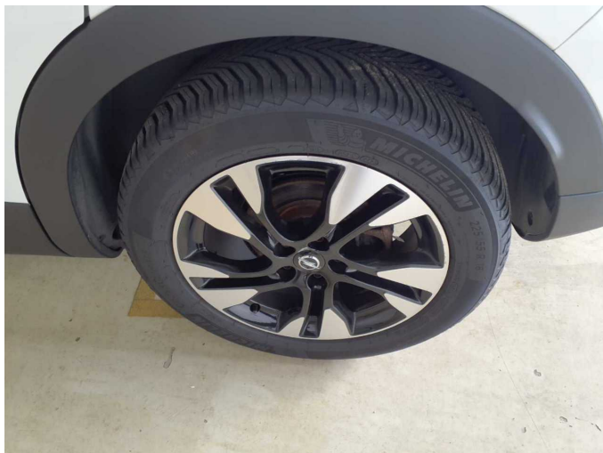
Damage 6: Wheel / tyres: Alloy rim - rear left side - Corrosion - Loss in value
