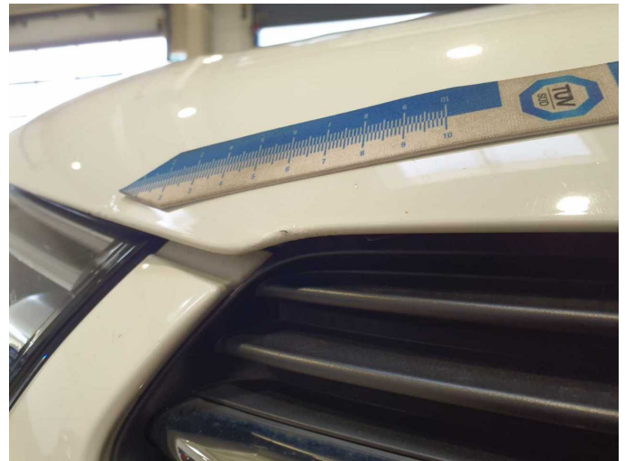
Damage 8: Bonnet: Bonnet - Corrosion - Repair and paint
