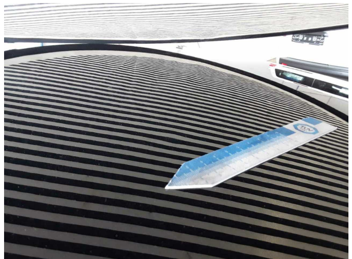
Damage 1: Roof: Roof - dent(s) - Smooth repair work
