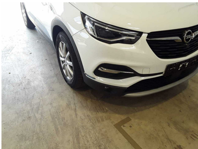
Damage 2: Front bumper: Spoiler - Differs from the original configuration - Un- / install
