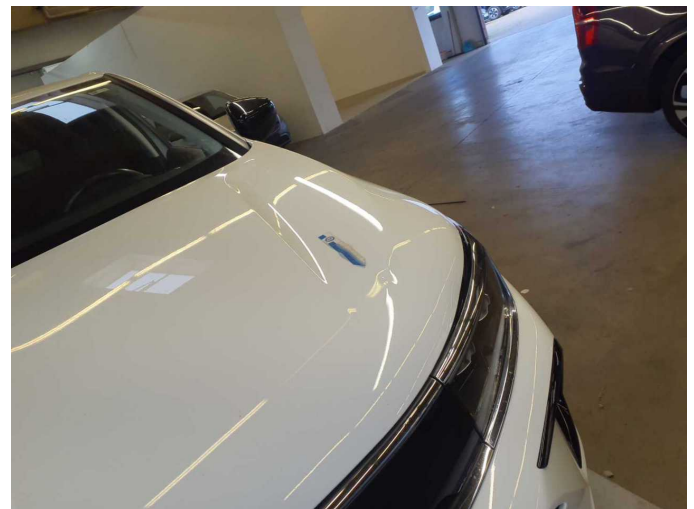
Damage 3: Bonnet: Bonnet - dent(s) - Smooth repair work
