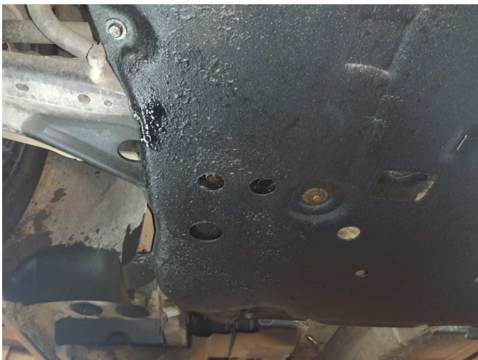
Damage 6: Engine: Engine (Motorraum-Unterboden Ölfeucht) - Leaking - Perform diagnosis
