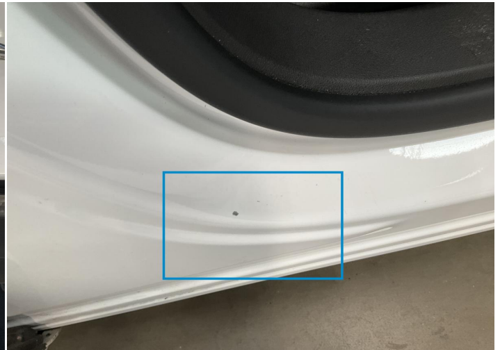
2. Pillar / Front Right Paint / Scratch / Scuff -
