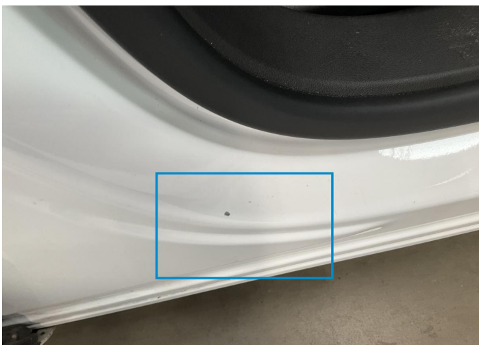
2. Pillar / Front Right Paint / Scratch / Scuff -
