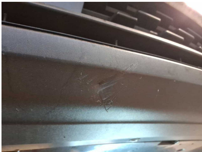
Damage 3: Front bumper: Spoiler - Deformed - Replace
