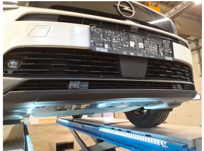
Damage 3: Front bumper: Spoiler - Deformed - Replace
