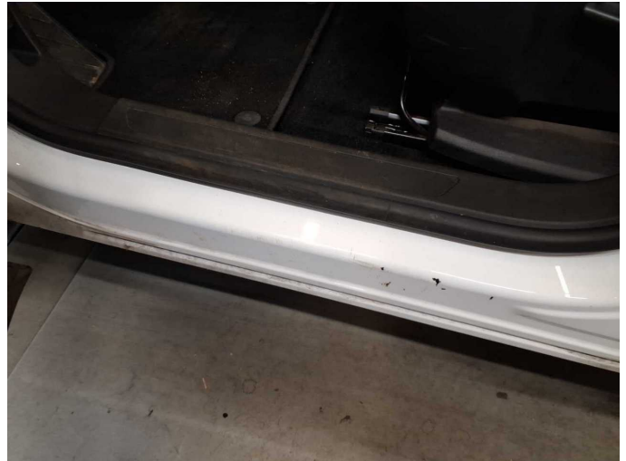
Wear and tear 1: Sill - left side: Sill - Scratch(es) - No deduction
