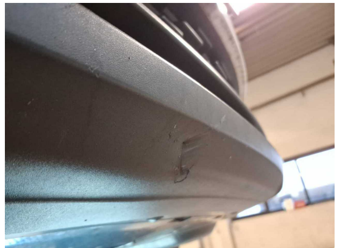
Damage 3: Front bumper: Spoiler - Deformed - Replace
