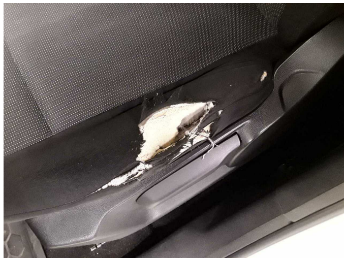
Damage 9: Seat - front: Seat cover - left side (inkl. Polster) - Broken / torn - Replace
