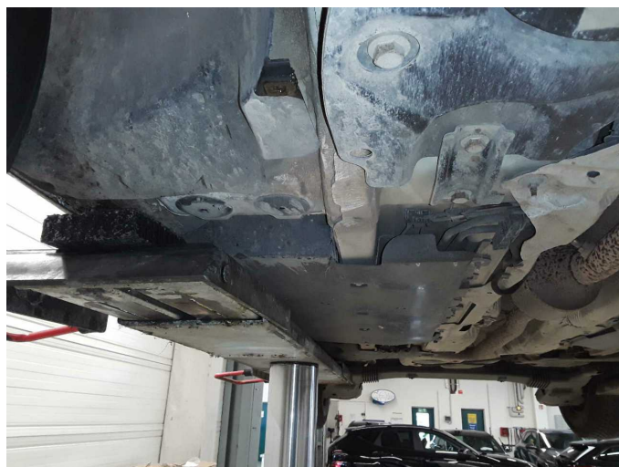
Damage 5: Body: Underbody panelling (Rechts) - Broken / torn - Replace
