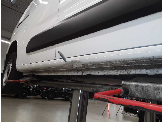
Damage 10: Sill - right side: Sill (Incl. Delle) - dent(s) - Repair and paint
