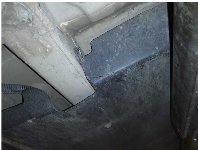
Damage 4: Body: Underbody panelling (Links) - Broken / torn - Replace
